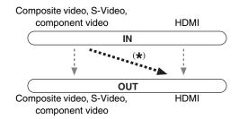
On the "Monitor Out" settings, you can select whether or not to have the video sources' images output through the HDMI output, as well as whether to have the onscreen setup menu output through the HDMI output or through an analog output.
